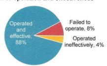
Sprinklers operated in 92% of the fires in which sprinklers were present and the fire was large enough to activate them.
