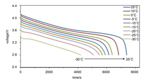
As one can see at the left hand side of the above graph, temperature effects battery voltage. And volts times amps equals watts. All chemical batteries are subject to lowering voltage as they are discharged, as well.
